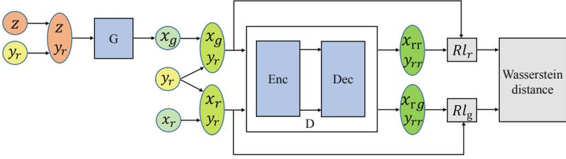
**Fig. 1.** Illustration of cBEGAN. cBEGAN adopts the auto-encoder to handle the difference between two reconstruction losses distributions. Here, G, D, Enc, Dec,  $RL_r$  and  $RL_g$  represent generator, discriminator, encoder, decoder and the two reconstruction losses, respectively.
